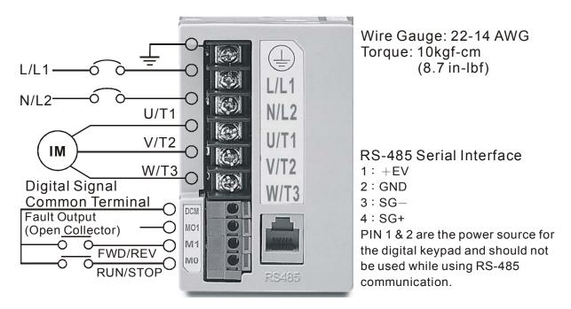
\*NOTE\*: Do not plug a Modem or telephone line to the RS-485 communication port, permanent damage may result. Terminals 2 & 5 are the power sources for the optional copy keypad and should not be used while using RS-485 communication.
