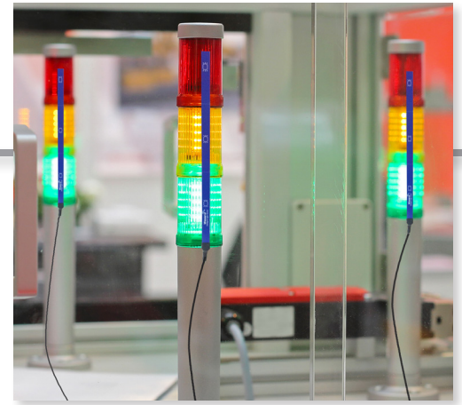
Stack light sensing, monitoring & reporting application
